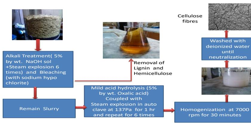
Figure 3 Extraction of CNF
