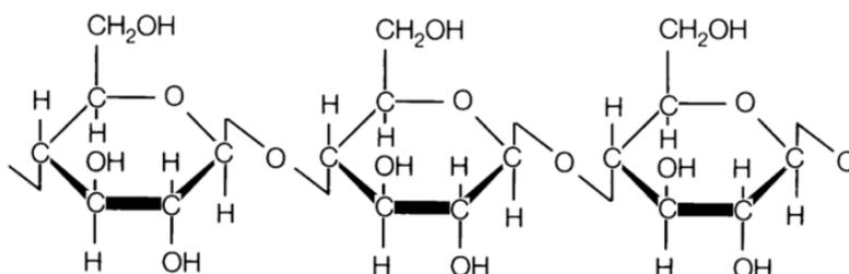
Figure 1 Structure of cellulose
