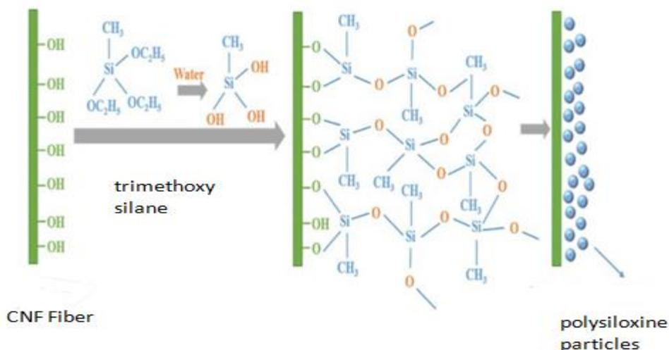
Figure 5 Chemistry of silination
