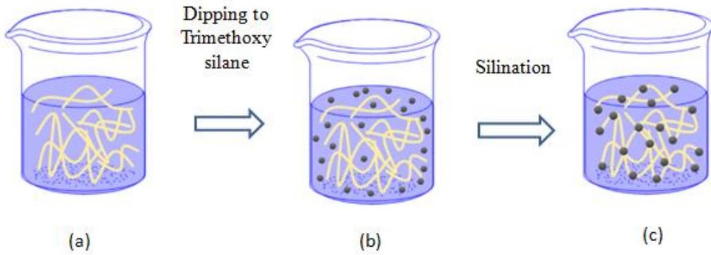
Figure 6 Morphology before and after silination
