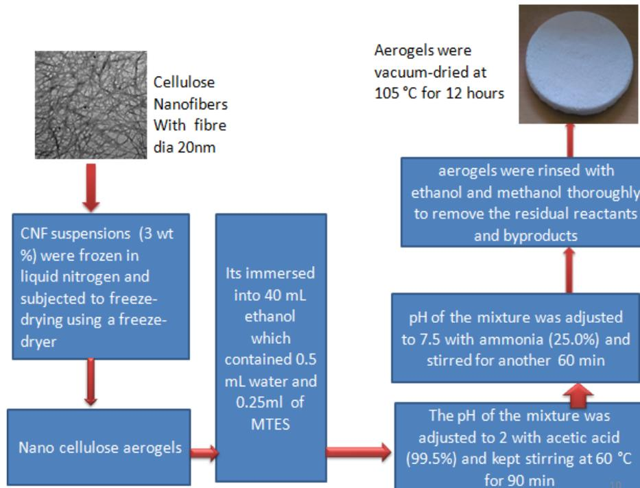
Figure 4 Silination of CNF aerogel
