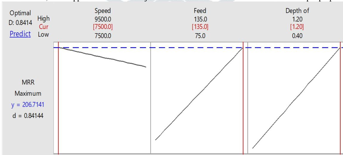
**Fig. 4: Optimized result for RSM technique**
