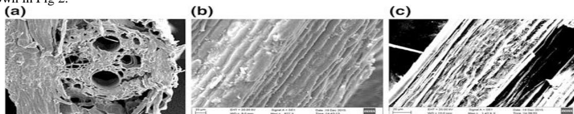
[Fig.3 Scanning electron microscope images ( a ) Cross sectional image of Sabai grass fibre ( b ) Sabai grass scoured Bleached SEM1 (c ) Sabai grass SEM1<sup>[7,8]</sup>
