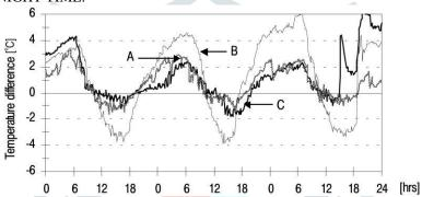
At night, outdoor air is allowed in and condensation may occur when the temperature of the metal roof becomes lower than the dew point temperature of the ambient air due to radiant cooling.
