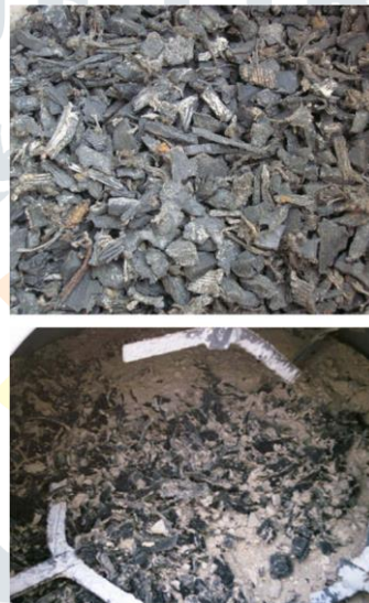
Fig. 1 Rubber particles: (above) as they come after the shredding process; (below) during the mixture of concrete [18].
