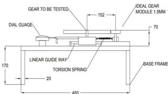
Fig. 2: Line diagram of Parkinson's Gear Tester [5]
