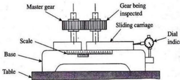
Fig. 1: Experimental setup of Parkinson's Gear Tester [1]
