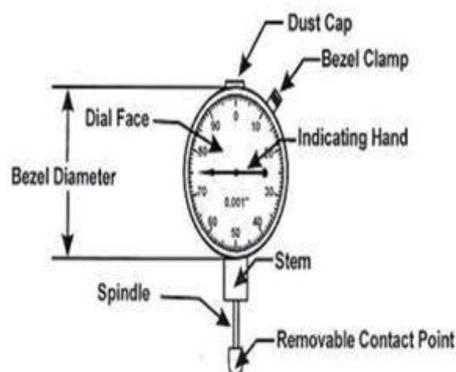
Fig 3: Specifications of dial gauge [5]
