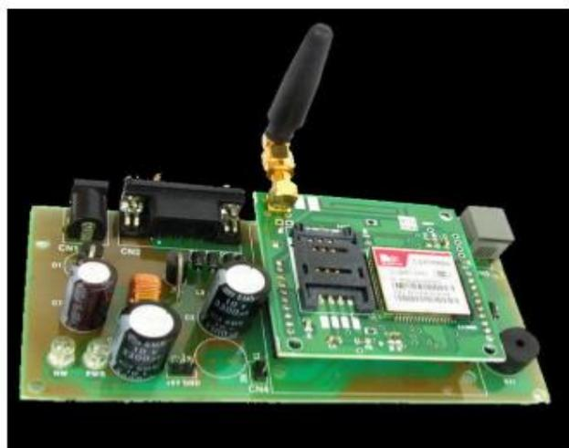
Fig-10: GSM modem
