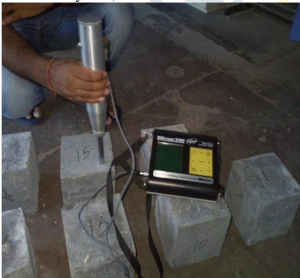
Rebound Hammer Test
