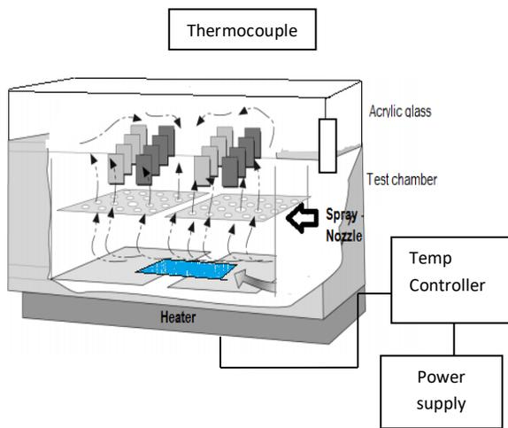
Fig. 1 Block Diagram of corrosion chamber
