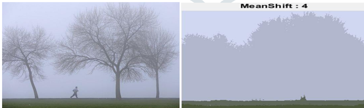
Figure: Segmentation results by mean shift algorithm, different regions are distinguished by different grey values
