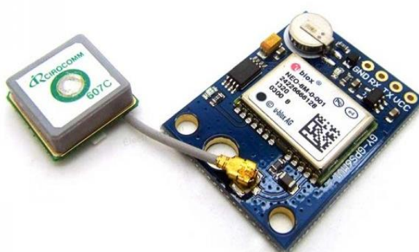
Fig 5: GPS Module with Active Antenna.
