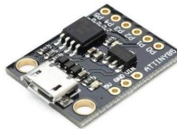
Fig 3: mini USB Board with ATtiny85 microcontroller
