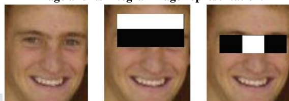
Figure 2. Examples of Haar features. Areas of white and black regions are multiplied by their respective weights and then summed in order to get the Haar feature value.
