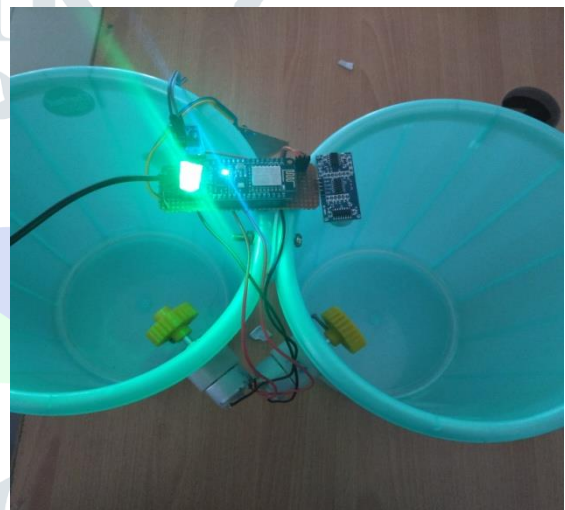
Fig:2-PTOTEUS FOR VACANT BIN INDICATED WITH GREEN LED
