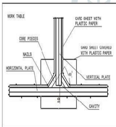
Fig.4 Experimental set up of Schematic T Joint.
