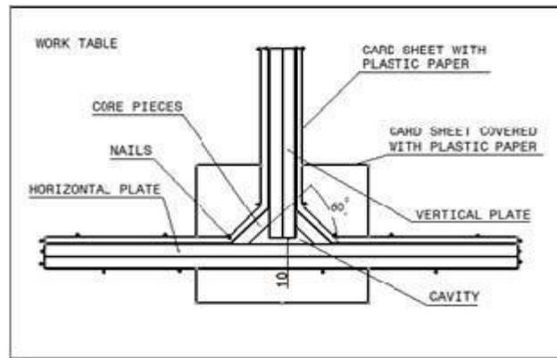
Figure 3 Typical mould arrangement for filler triangle.
