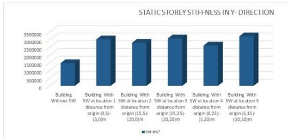
Static Storey Stiffness in Y-Direction (KN/M)
