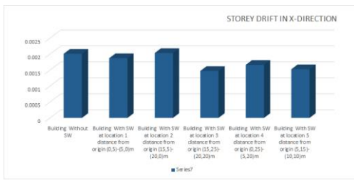
Static Storey Drift in X-Direction (Unitless)
