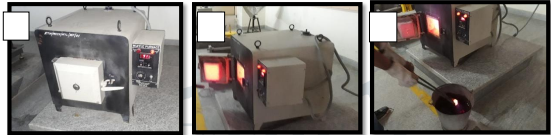
Figure 2 .(a) muffle furnace , (b) heat treatment process ,(c) quenching process.
