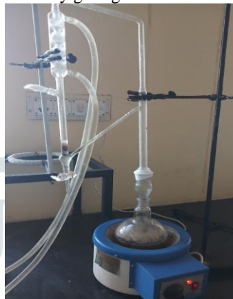
Fig 1: Experimental setup of Steam Distillation
