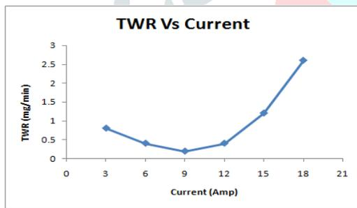
Fig. 4.7 Effect of current on TWR
