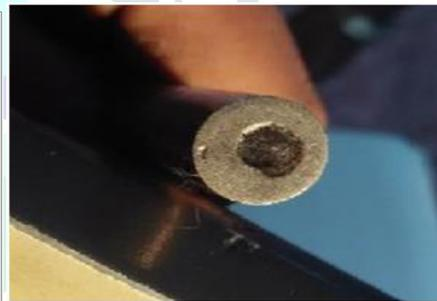
Fig.4.4 Melting of tool at 18 Amps.
