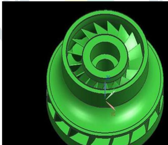
**Fig.3: Complete Assembly of 3D Shrouded Impeller**
