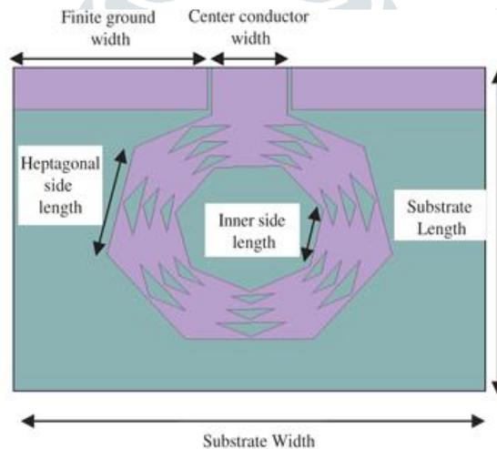
Fig. 3 Heptagonal shaped antenna
