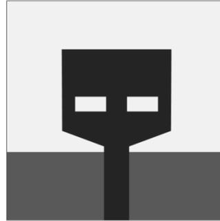
Fig.5 compact UWB wearable antenna
