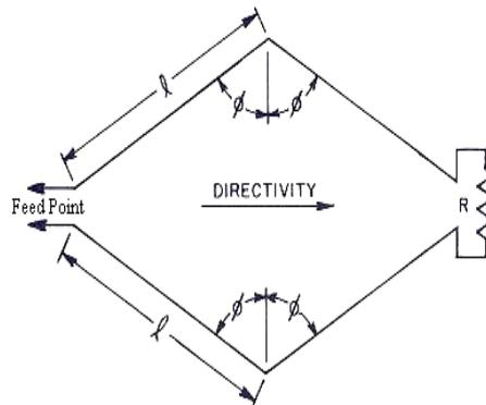
Fig.2 Diamond Shaped Textile Wearable Antenna
