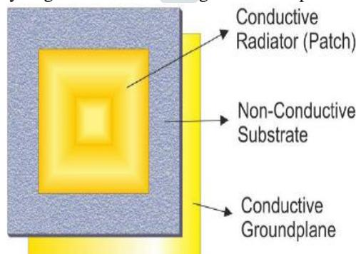
Fig .1 General diagram of on-body textile antenna
