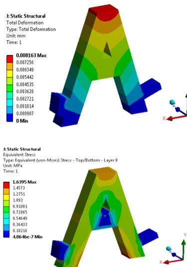
Figure.6.Case 3 deformation and equivalent stress
