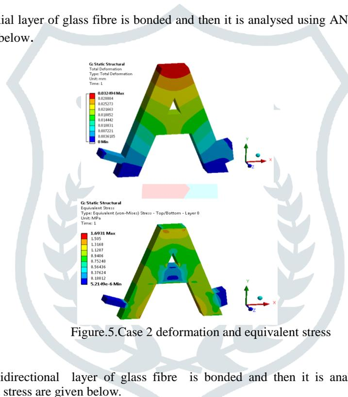
Figure.5.Case 2 deformation and equivalent stress
