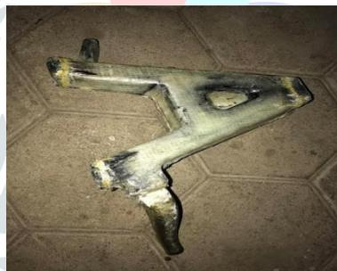
Figure.8.Glass Fibre centre stand
