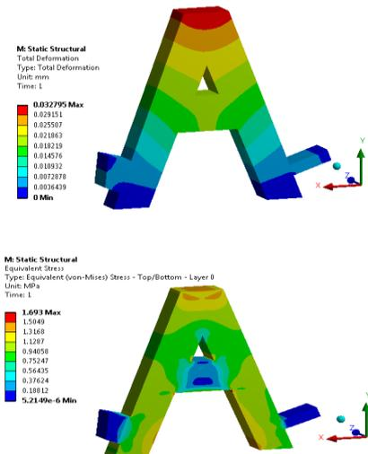
Figure.7.Case 4 deformation and equivalent stress
