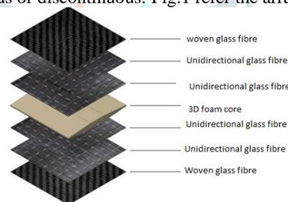
Figure.1. Arrangement of layers in composites
