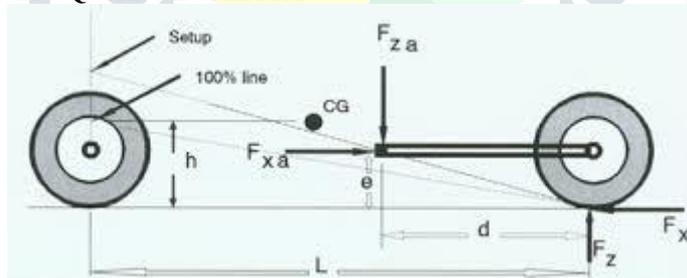
Anti-dive and anti-lift are tricks that can be applied to a truck's front suspension geometry to control brake drive and acceleration lift
