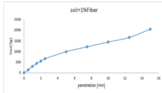
Figure 4.20: Soil reinforced with 1% of coir
