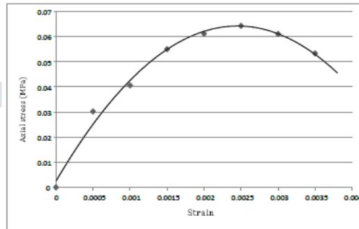
Figure 4.15: Soil reinforced with 1% of coir
