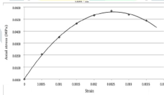
Figure 4.12 soil without reinforced
