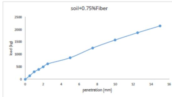
Figure 4.19 soil reinforced with 0.75 % coir
