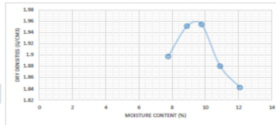
Figure 4.3 Soil + 0.5% coconut coir fibre
