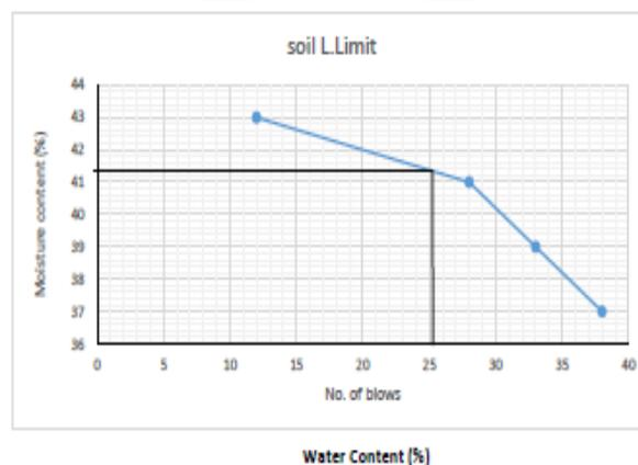
Figure 4.1 liquid limit for soil
