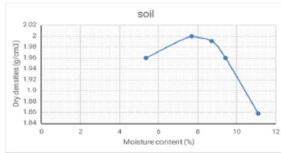
Figure 4.2 soil without reinforcement
