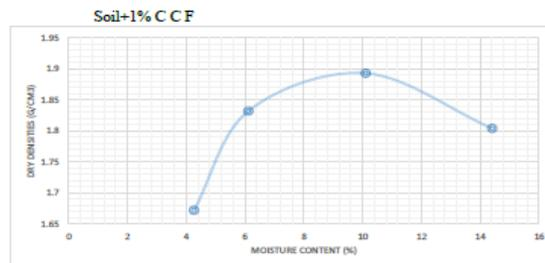
Figure 4.5 Soil + 1% coconut coir fibre
