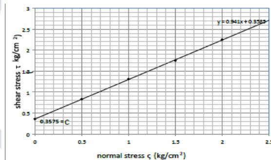
Figure 4.8 soil reinforced with 0.5 % coir
