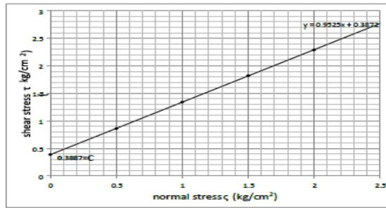
Figure 4.10: Soil reinforced with 1% of coir
