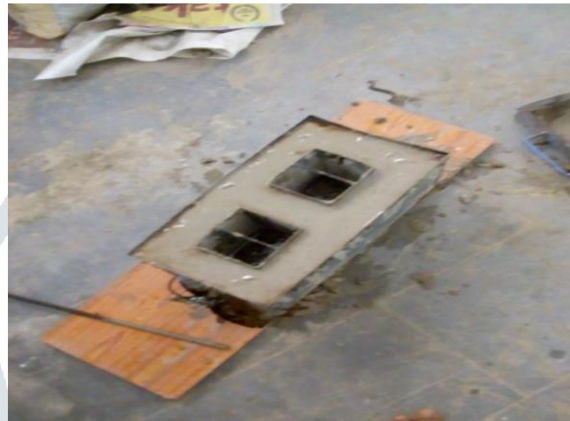
Figure 4.1 Hollow Block Cube of 400x200x200mm Size
