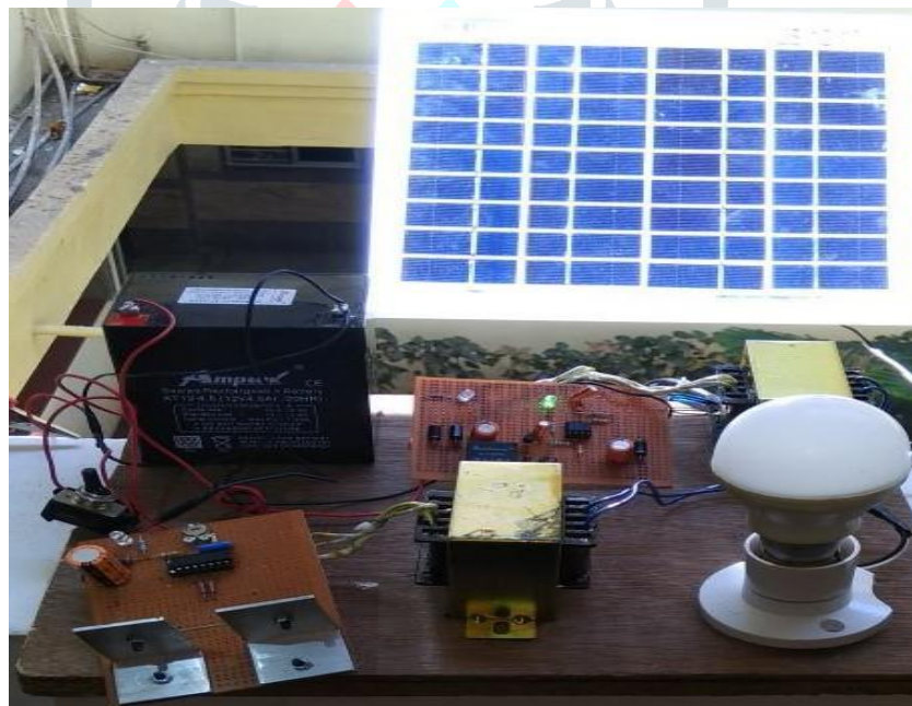
Fig 5.4 Hybrid inverter with solar battery charging circuit while charging with solar power
