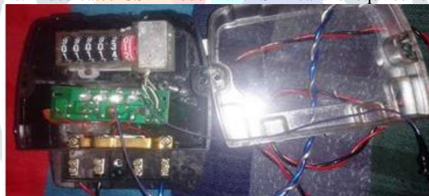
Fig.3. Connection of Arduino with Energy Meter
