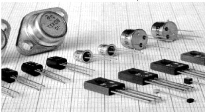
A voltage or current applied to one pair of the transistor's terminals changes the current flowing through another pair of terminals. Because the controlled (output) power can be much more than the controlling (input) power, the transistor provides amplification of a signal. Today, some transistors are packaged individually, but many more are found embedded in integrated circuits.
