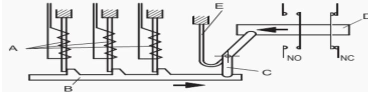
**Fig 2.1(e)** Principle of operation of a three pole thermally delayed bimetal motor protection relay with temperature compensation.
