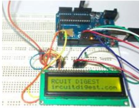
Fig: 16x2 LCD Interfacing with Arduino Uno
