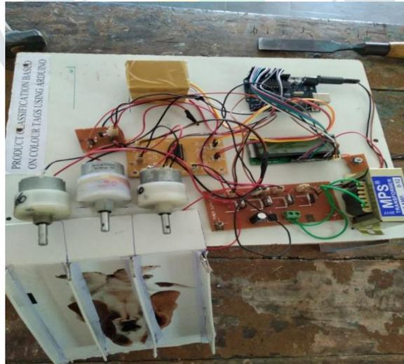
In this paper, we can identify the color by placing the color tags in front of the color sensor and after detecting the color the corresponding motor will rotate.
