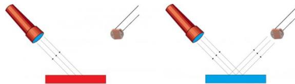
Similarly, when a bright blue light is incident on both the objects, the blue object will appear the brightest to the sensor. This method is just to understand the working of a color sensor and the actual results may not be accurate.
