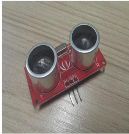
Fig 2: Ultrasonic sensor
