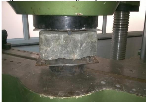
**Fig No 6: cross sectional view loading test specimen for flexural strength**
