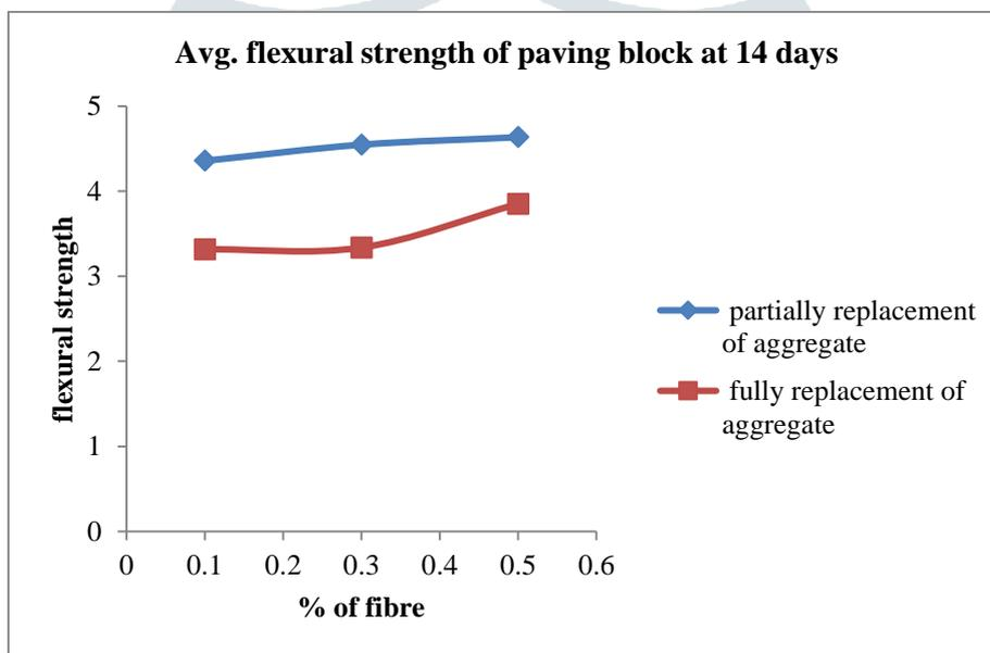
Fig No 8: Average Flexural Strength of paving blocks at 14 days.
