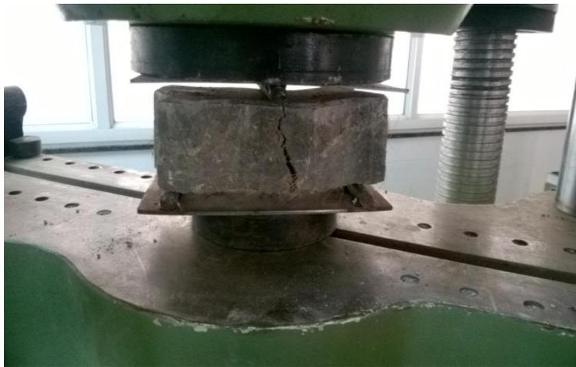
Fig No 7: failure of specimen during Flexure Strength Test
