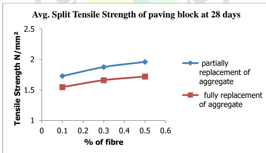
Fig No 12: Average Tensile Strength of paving blocks at 28 days.
