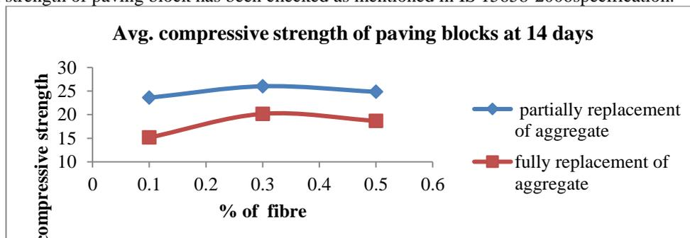
**Fig No 2: Average Compressive strength of paving blocks at 14 days.**
