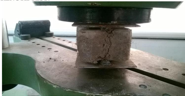
Fig No 10: Split tensile Strength Test Setup
