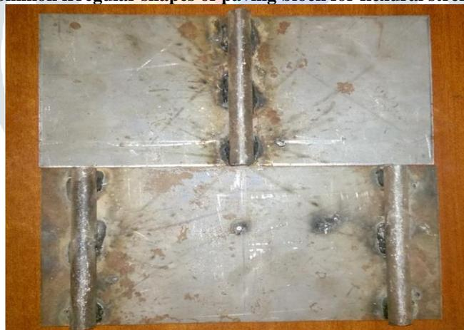
**Fig No 5: longitudinal view of loading test specimen for flexural strength**
