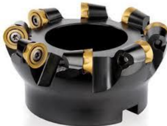
Fig. 6 Face mill tipped with carbide inserts
