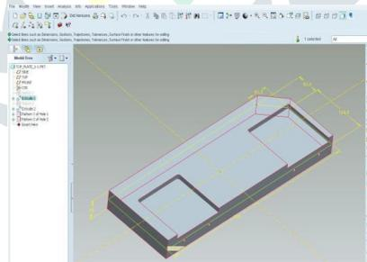
Fig. 4. Support Plate for the Base Frame Assembly
