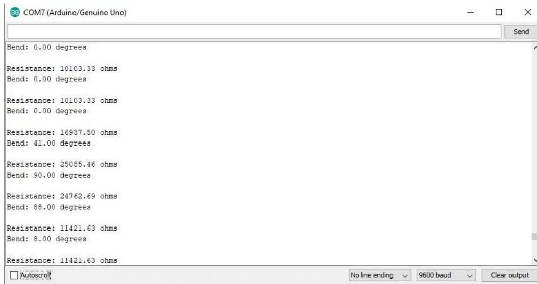
Figure 5 Flax Sensor Banding Angle Output
