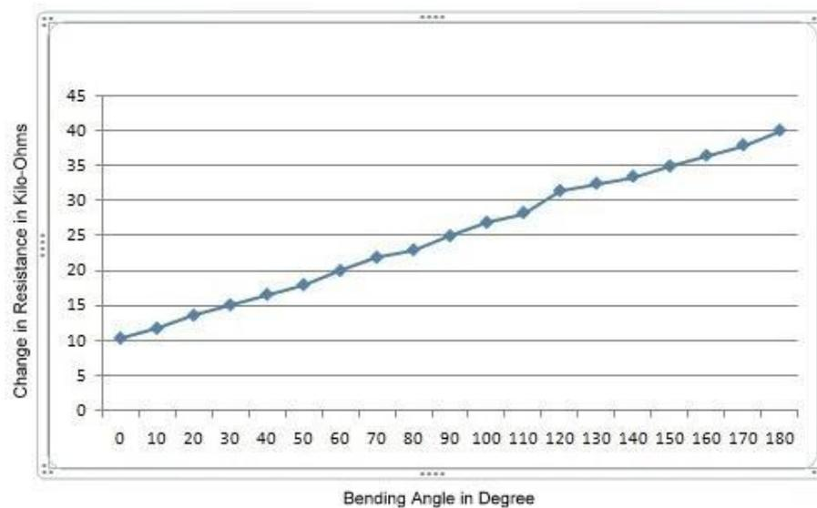
**Figure 6** Graph – Bending Angle v/s Resistance
