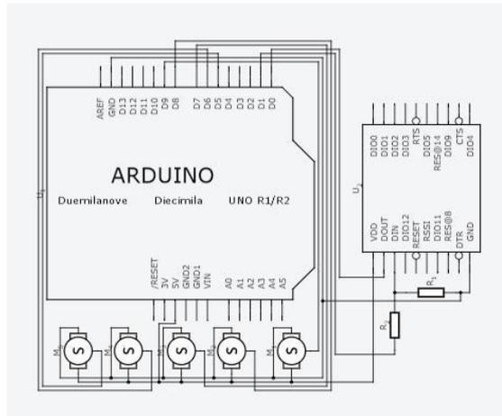
Figure 4 Circuit Diagram of Robo Hand
