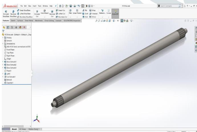
Fig.2 Cad model of Drive Axle
