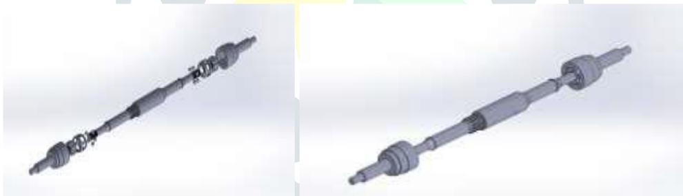
Fig.1 Assembled View of Drive Axle <sup>[1]</sup>
