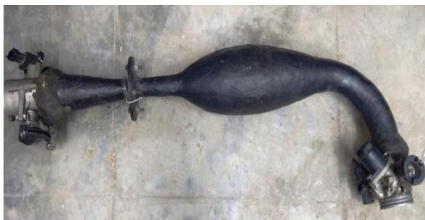
Fig 1 Intake System of GTM 17
