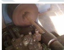
Figure 10: Facing operation (left), turning operation (right) with Lathe Machine.
