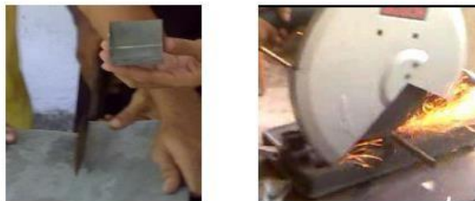
Figure 4: Cutting Sheet metal with sniping tool (left), shaft with Grinding C
