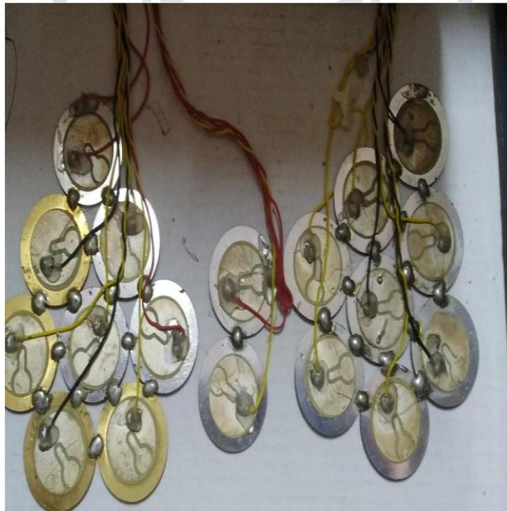
Fig. 5. Piezo discs parallel connections
