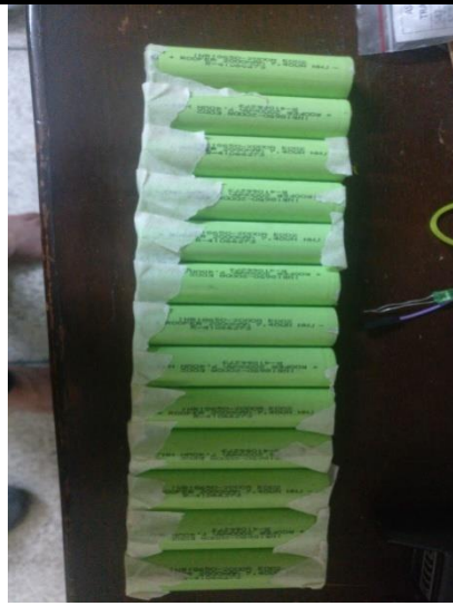
Fig2: Li-ion battery 13s-1p
