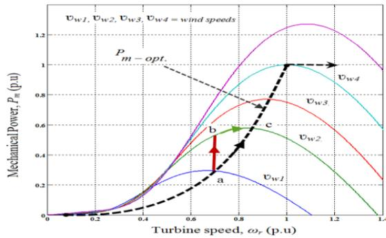
Fig. 3 Optimum Power Curve or Optimum Power Line
