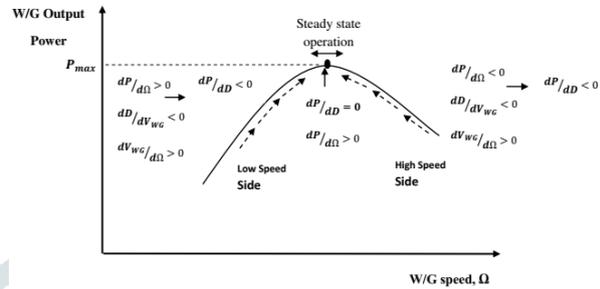
Fig. 4 MPPT process of WG
