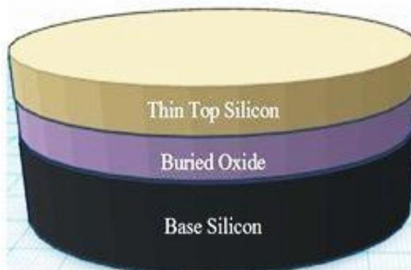
Fig.5 SOI wafer layers
