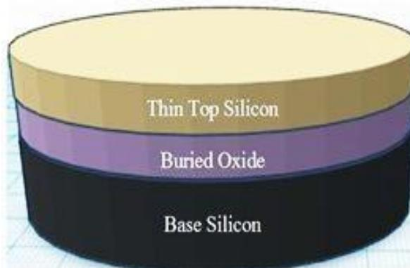
Fig.5 SOI wafer layers
