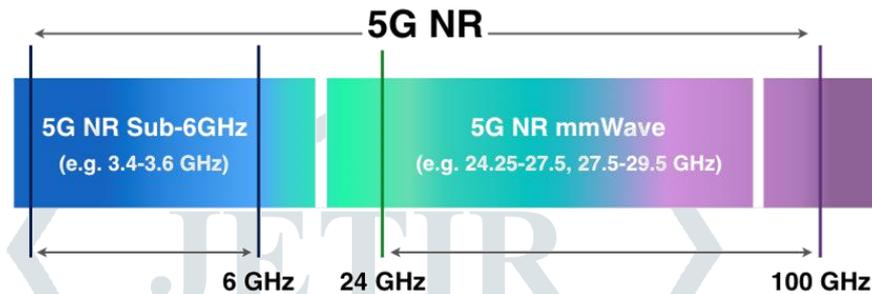
Fig. 1: 5G New Radio unified design across diverse spectrum bands and types including Millimeter Wave spectrum [7].
