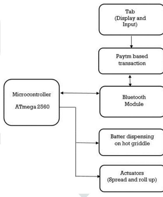
**Microcontroller:** The controller used is ATmega 2560. It has all the functional requirements required for this application.
