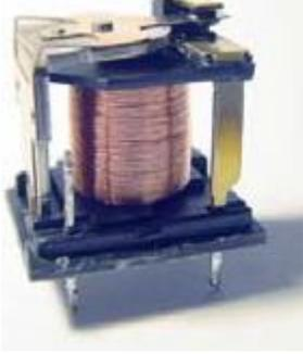
**Fig 4 Relay Basic Section**
