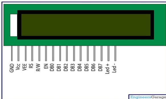
**Fig 5 Pin Diagram of LCD**
