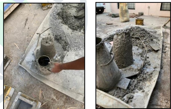
Fig no 2 Slumps of various concrete mixes
