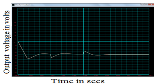
Fig 7 Closed loop response of NOELC with ZN-PI controller under sudden line disturbance from 10V - 12 V (20%) at 0.003 sec and 10V - 8V(20%) at 0.006 sec.
