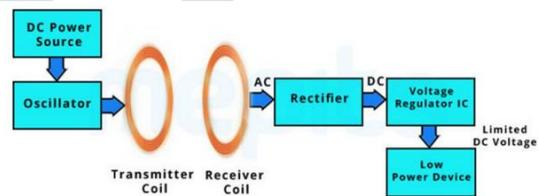
Fig.3.wireless power transmission
