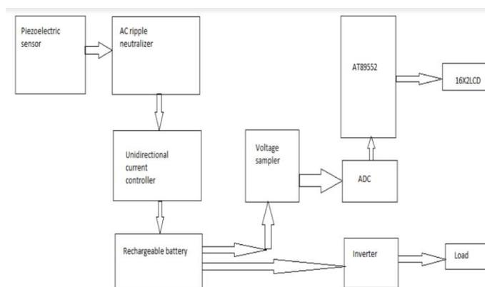
Fig .2. footstep power generation
