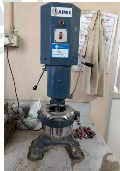
Fig. 1: Planetary Mixer used for mixing
