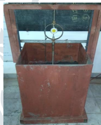
Fig. 4: Testing tank with loading arrangement
