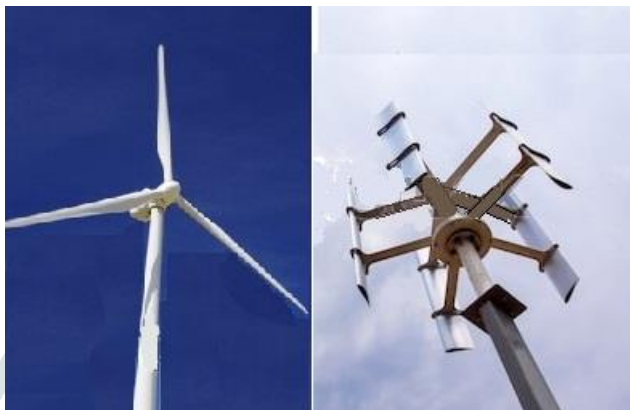
Fig. 1: Horizontal axis wind turbine and Vertical axis wind turbine (Source: Shutterstock)
