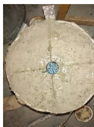
Fig. 2: horizontally reinforced granular column
